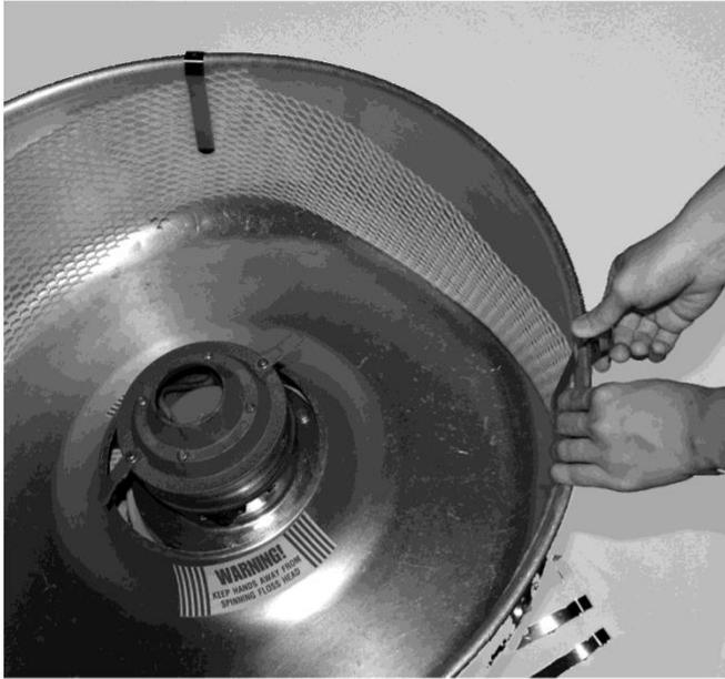
Using the five metal clips provided, attach the plastic mesh stabilizer to the inside of the floss pan. Pull the mesh gently to create a space between the mesh and the pan
